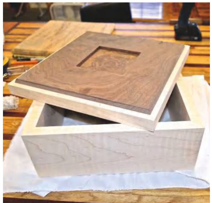
▲ Pic.9 After the glue had set, I ran the box on its four sides through the table saw, 25mm from the top to release the lid from the carcass. Now there were two pieces
